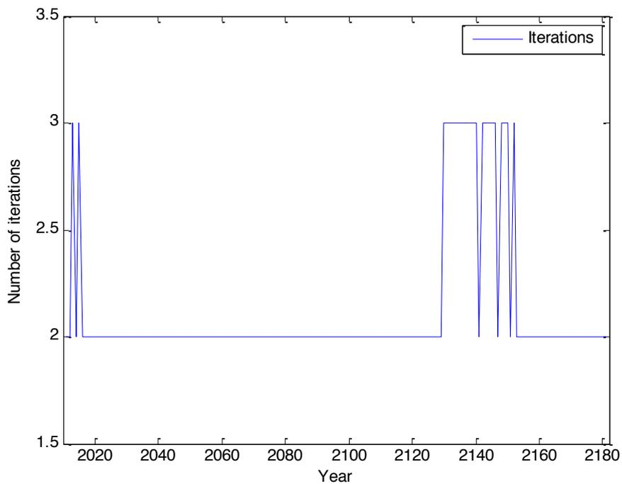
Figure 1 Number of iterations completed for a convergence tolerance level of 10%
